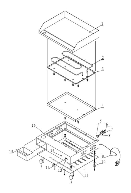
Exploded diagram and spare parts list L515 Rev.2
