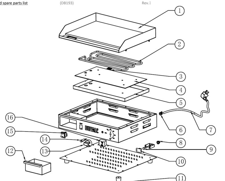
Exploded diagram and spare parts list (DB193)
