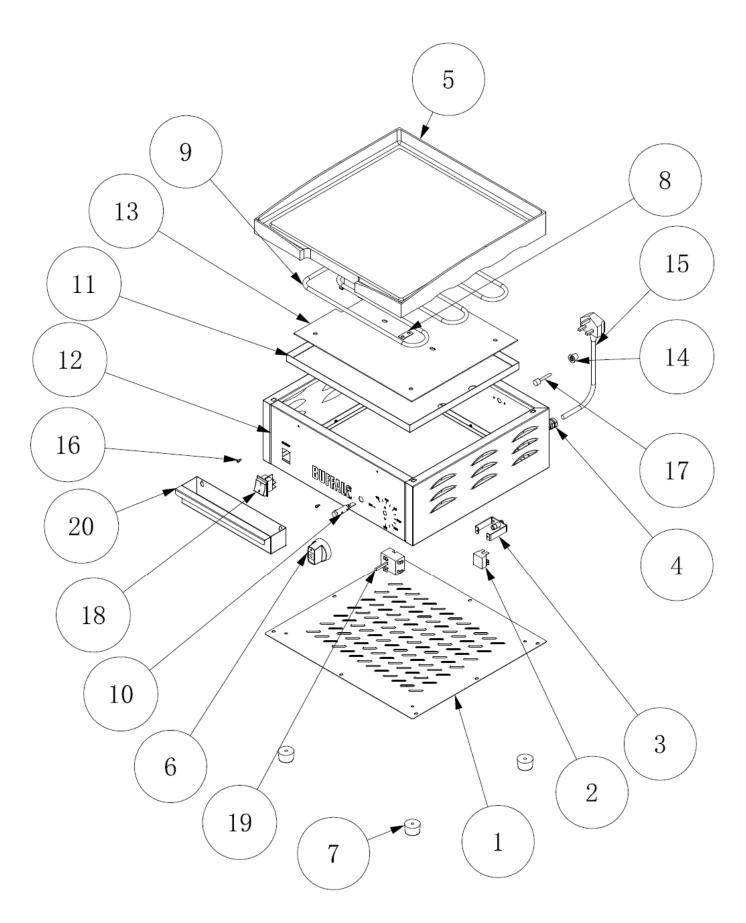
Exploded diagram and spare parts list (DC901)
