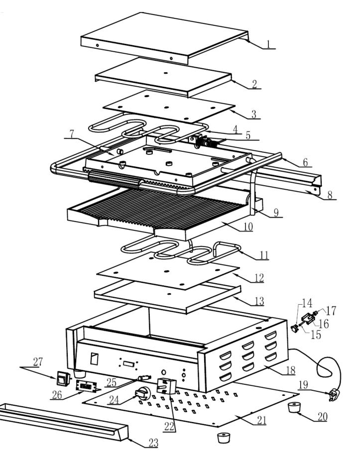
Exploded diagram and spare parts list (FC380)
